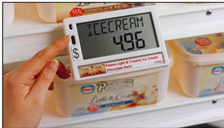
The lid electronic shelf labelling system is designed to get price information simultaneously identical on shelves and at checkouts right across a chain of supermarkets.
